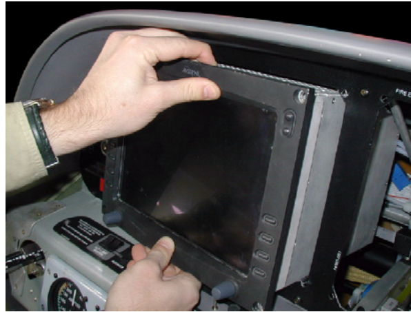
Figure 5 – PFD Handling When Installing
